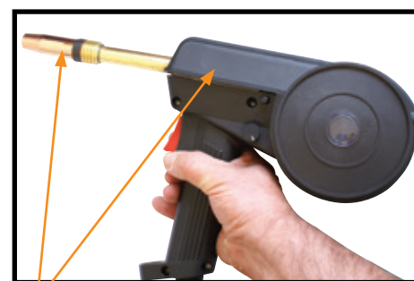
(14) Fit the gas nozzle and close the wire feed spool cover
