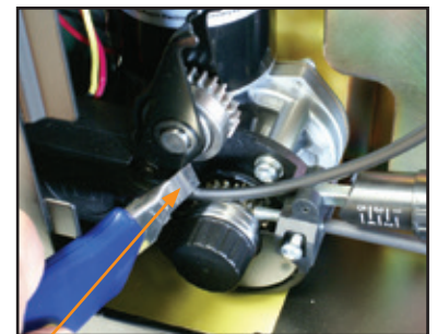
(15) Cut the extended Polymide liner with a sharp Stanley knife just in front of the drive roller
