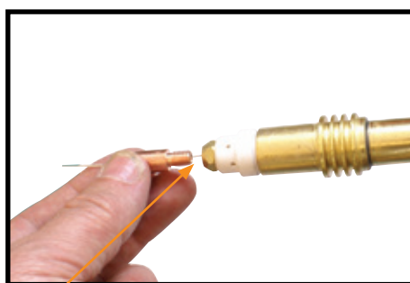
(13) Fit the contact tip over the wire and screw it into the tip holder, nip it up tight.
