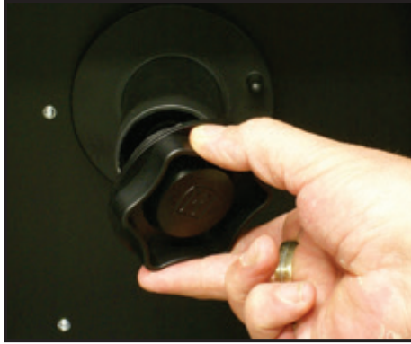
(1) Remove the spool retaining nut.
