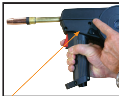
(7) Push the cover release button to unlock the wire feed / spool cover
